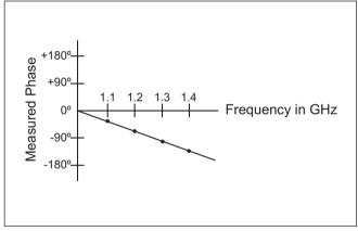
Figure 10. Electrical Delay
