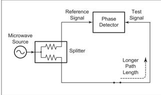
Reference Test Signal Signal Phase Detector Microwave Source ∿₩ Splitter w Longer by , One Wavelength Length (360 Degrees)
