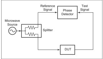
Figure 6. Splitting the Microwave Signal
