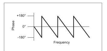
Figure 16. Linear Phase with frequency Waveform
