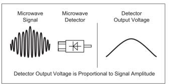
Figure 3. Scalar Analyzer Detection
