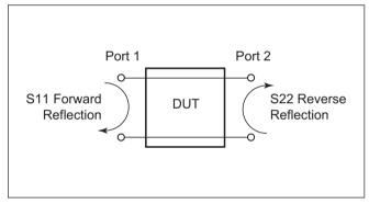
Figure 14. Forward and Reverse Measurements
